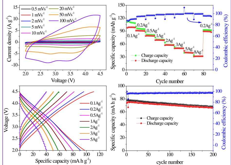
The incorporation of carbon nanotube (CNT) give rise to much enhanced capacitance of activated carbon
