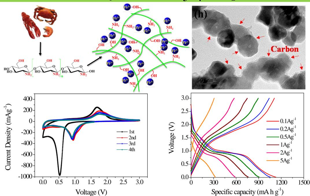
$\text{Fe}_3\text{O}_4$  with excellent battery performance was prepared by utilizing the correlation of metal ion with amino and hydroxyl groups of biomass material (chitosan)
