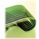
研發新型的薄膜有機太陽能電池,輕薄可捲曲及能做成 半透明,效能達世界最高的11.5%,並獲美國能源部國 家再生能源實驗室 (NREL) 正式確認為主要科技突破,並 刊登於國際知名的「最佳效能研究電池圖表」上。 Developed a new type of thin film organic PV, light weight, bendable and can be semi-transparent, with a record efficiency of 11.5%, which has been officially certified as a major technological breakthrough in the renowned National Renewable Energy Laboratory (NREL) (US Dept of Energy) chart of "best research-cell efficiencies".
