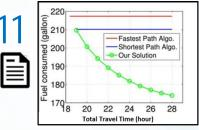
團隊設計的高效能演算法能為重型卡 車節省高達 17% 油耗,同時滿足運輸 期限的要求。The highly-efficient algorithm solution is able to reduce the truck's fuel consumption by up to 17%, while meeting the deadline constraint.
