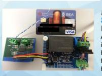
成功研發本港首個智慧型電氣負載控制 器之理論設計及硬件製作,能應用在不 同家居電器,回應電網頻率或電壓變化 A first of its kind smart demand controller in HK (both theoretical design and hardware implementation) enabling frequency/voltage response from various home appliances.
